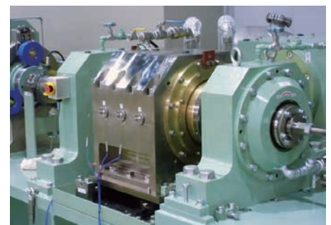
Test Equipment of 300mm shaft Dia.
