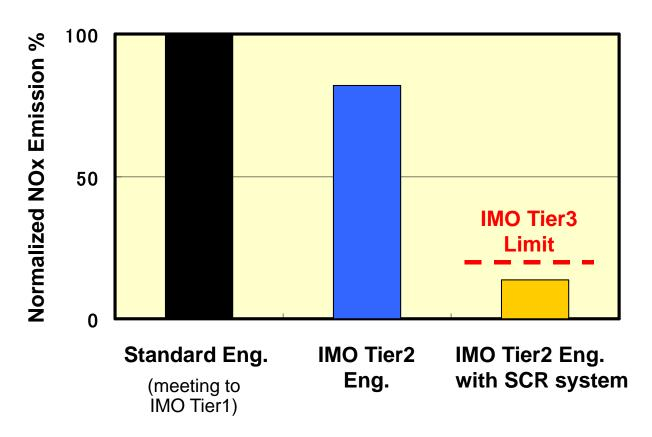
• SCR was fitted with a Tier II compliant engine. As a result of this laboratory test conducted at SV = 20000 h<sup>-1</sup>, 80% denitration rate required by Tier III was achieved.
