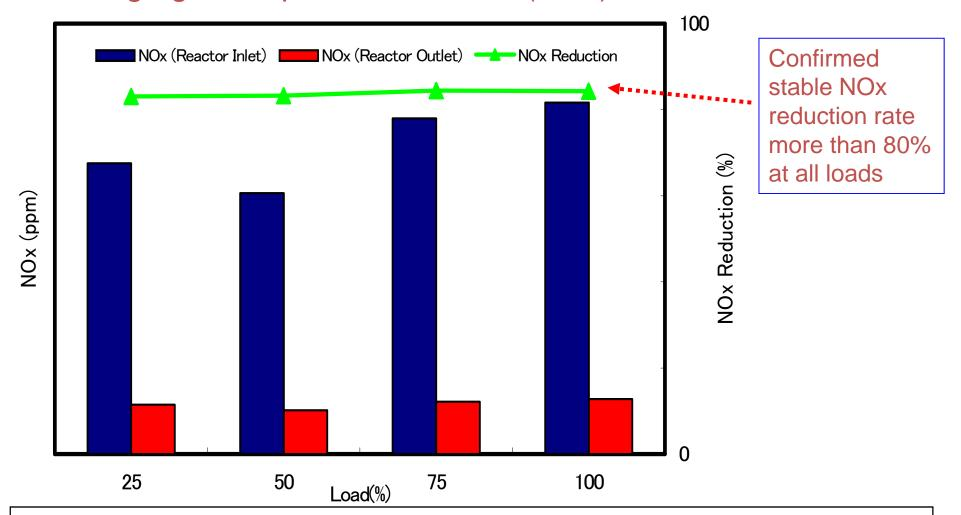
SV number was kept between 2500 and 2600 which is within the harmless level to the function of SCR system.
